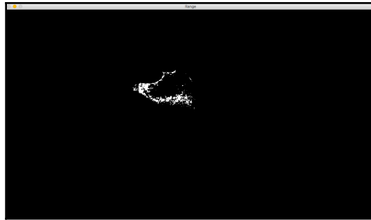
Figure 2: The output of the inRange() function used to find the region within the pixel value bounds
