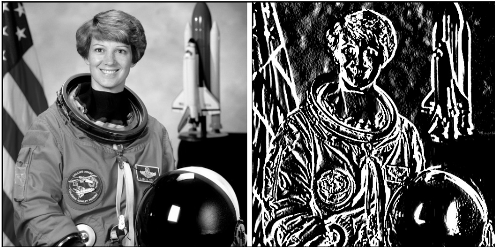
Figure 13: The image on the left is the input image and the image on the right is the output of Sobel in the x direction
